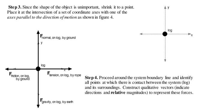
**Step 5:** Indicate which forces (if any) are equal in magnitude to other forces. The problem states that the tractor pulls the log at constant velocity, so we know that the net force has to be zero. In other words, the forces up must equal the forces down, and the forces left must equal the forces right. In the diagram below these equalities have been marked with hashes like those used to indicate congruences in geometry.
