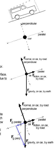
In each of the following situations, represent the object with a particle. Sketch all the forces acting upon the object, making the length of each vector represent the magnitude of the force. Also use congruency marks to indicate which vectors are equal in magnitude.
