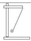
Experiment #2: Angle of swing - amplitude (the angle between the rest position and where the end of the swing is located.)
